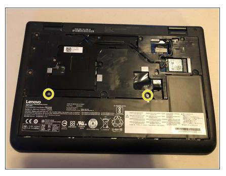
There will be 2 other Philips screws under the cover there should also be two arrows pointing at each screw that needs to be removed.
