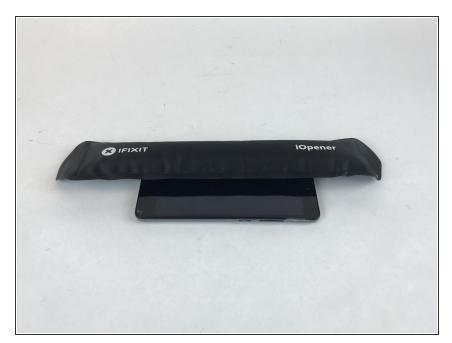
To prepare the iOpener insert it in the microwave for 30 seconds and apply it on the side edges of the phone so that the glue underneath will soften.
