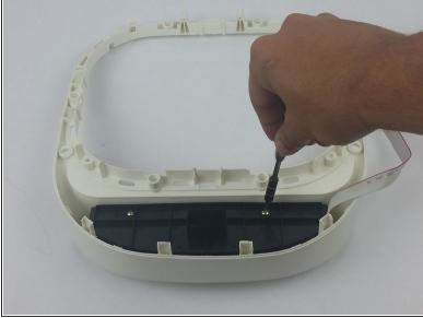
Remove the two 11mm Phillips #1 screws from the top cover.
