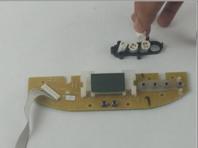
Remove and replace buttons as necessary.
