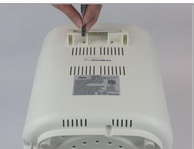
Remove the two 11mm Phillips #1 screws from the back of the device.
