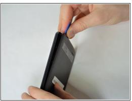
Start at one corner, and use the plastic opening pick from the iFixit kit to wedge underneath the
