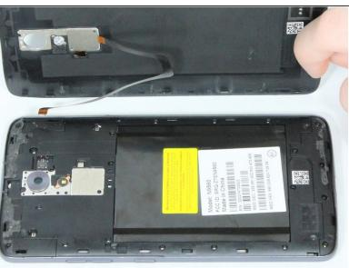
After removal of the two 3.4mm JIS #00 screws, disconnect the connector that attaches the ribbon wire from the main part of the phone.
