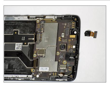
With the metal connector detached, the camera is fully disconnected from the phone and ready to be replaced.
