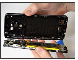
Use a plastic pick between the screen and side trim battery cover to remove the screen.
