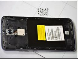
Remove the nineteen 3.4mm JIS #00 screws on the perimeter of the back using the JIS #00 screwdriver.
