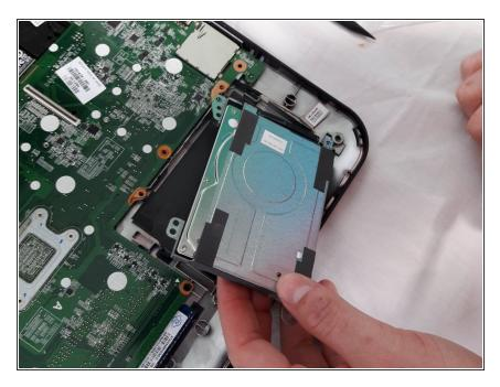
Remove hard drive from bracket being careful of it's cable.
