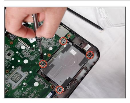
Remove the 4 x 5.5 mm screws connecting the hard drive tot he case.
