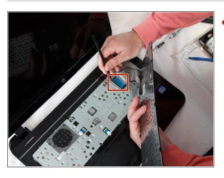
Remove keyboard wire by popping latch under blue plastic
