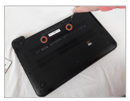
Remove the two 6.5mm Phillips #1 keyboard screws from bottom of laptop.
