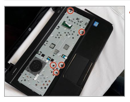
Remove the five 5.5mm Phillips #1 screws from the case
