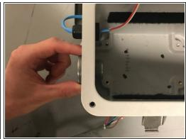
(i) Put the connector piece into the node (may have to hold it in place for the subsequent steps)
