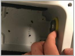
(i) Pull the yellow seal over the inside of the connector piece
