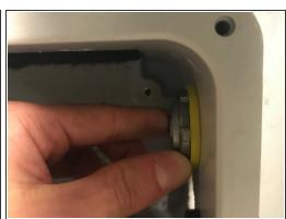
(i) Screw the tightener piece onto the connector
