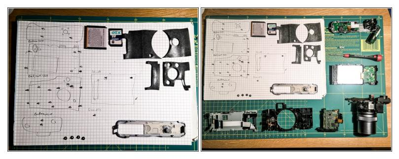
Two pictures showing a) the parts and b) the screws and their position.
