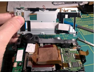
Finally! You can move the steel part away and by opening the last remaining FPC connector on the main PCB you can remove this steel thing completely.
