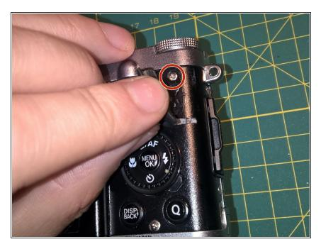
Remove the screw hiding below the rubber-pad.
