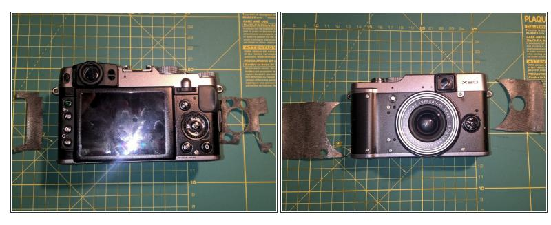
Remove four pieces of leatherette from the front and the back of the camera. Lift the edge of the leatherette and pull. The material itself is quite sturdy and the glue will still be good if you re-apply the pieces after you are finished.
