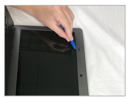
Separate the front bezel from the display using the plastic opening tool.
