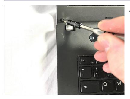
Remove the two 2mm Phillips #00 screws found at the bottom corners of the display.
