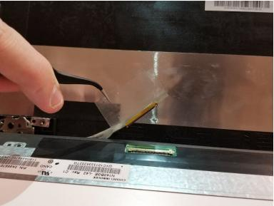
Peel up the adhesive tape to unlatch the metal retaining bracket on the display cable.
