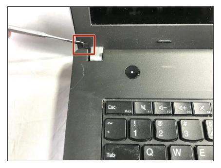
Use the pointed end of a spudger to remove the two screw covers from the bottom corners of the display.
