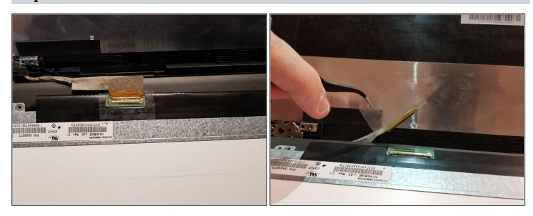
• Peel up the adhesive tape to unlatch the metal retaining bracket on the display cable.
