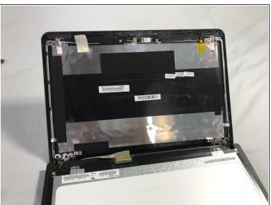
Lay the screen flat on top of the keyboard.
