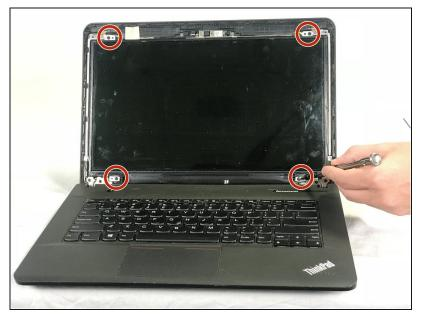
• Remove the four 2mm Phillips #00 screws from the screen.
