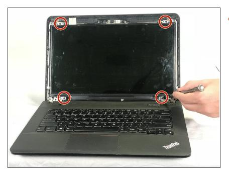
Remove the four 2mm Phillips #00 screws from the screen.
