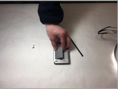
• Insert the nylon spudger into the battery cover release slot to remove the battery from the device.
