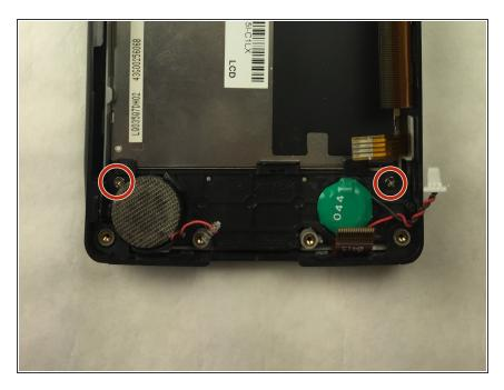
Remove the two 9.6 mm screws by the speaker and green battery with a JIS #0 screwdriver.
