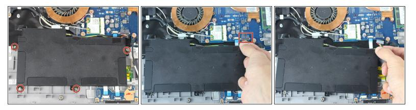
Use the screwdriver to remove the four 3.5mm long screws holding the battery in place. Then
