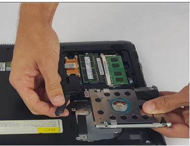
Unplug the connector from the hard drive by pulling straight out.
