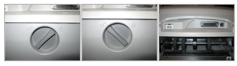
Remove the paper jam door from the printer by turning the dial from the locked position to the unlocked position.
