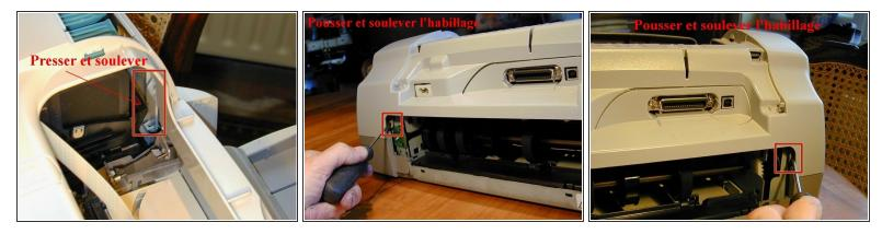
Push and lift the tabs shown with a flat-head screwdriver.
