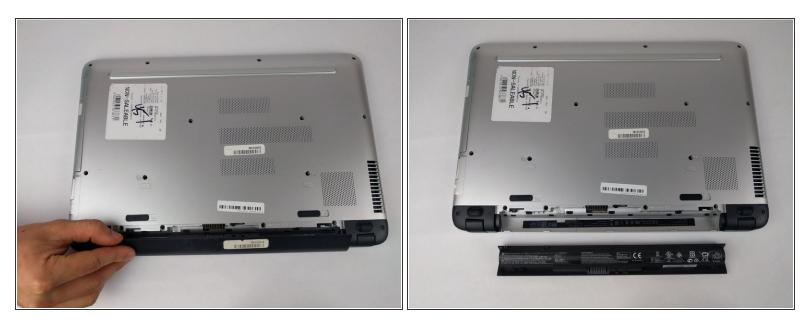
• Grabbing the top edge of the battery, rotate it toward you and then lift upward to relieve the battery from its slot.
