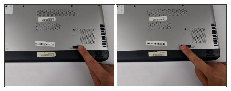
• Slide the battery lock tab toward the center of the battery to the unlock position.
