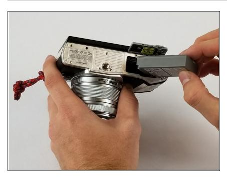
You can now remove the battery from the body of the camera and begin reassembly with your new battery.
