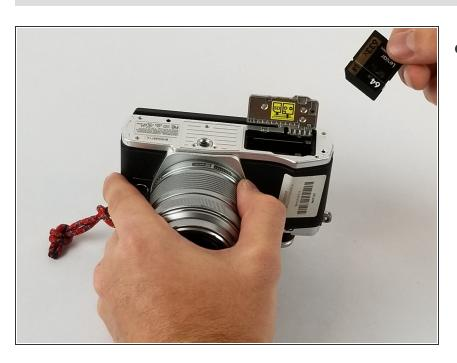
Remove the SD card from the camera by grabbing it with your fingers and lifting away from the camera.
