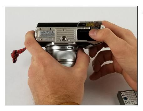
Find the SD card located near the hinges of the door and gently press down on it so that it becomes free.
