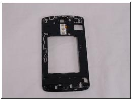
Remove the buttons frame on the back side the shield, by inserting a plastic opening tool underneath the frame.
