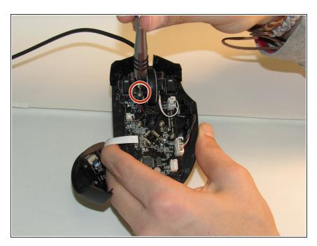
Using a Phillips #00 screwdriver, remove the 5mm screw holding the scroll wheel in place.
