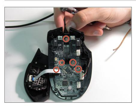
Using a Phillips #00 screwdriver, remove all five 5mm screws that connect the motherboard to the main frame.
