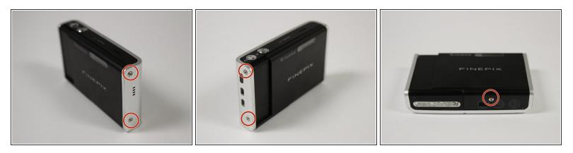
• Open the camera by removing the 5 external 4.0 mm screws with the 1.0 flathead.
