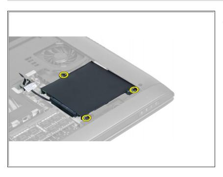
Remove the screws that secure the hard drive to the computer.
