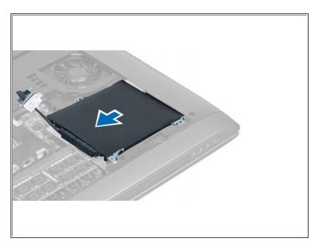
Slide and remove the hard drive from the computer.
