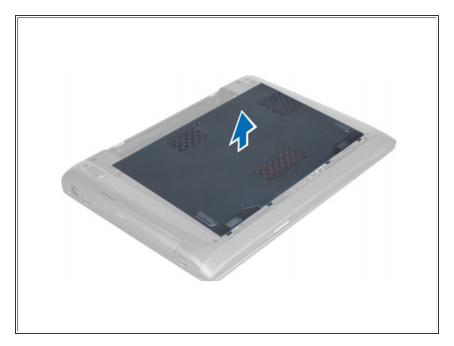
Lift the cover upwards and away from the computer.
