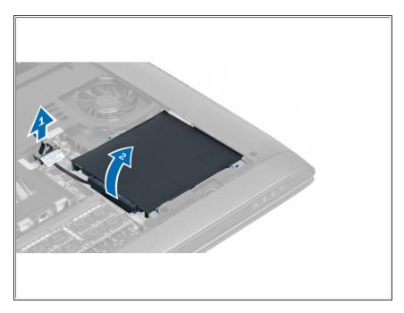
Lift the tab to disconnect the harddrive cable from the system board.
