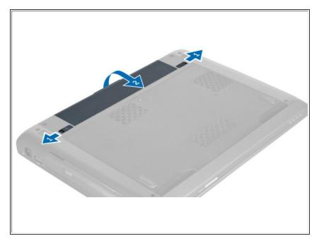
Slide the battery latches to release the battery.
