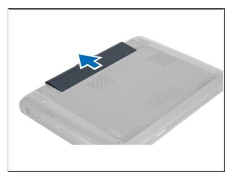
Lift and remove the battery from the computer.
