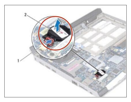
Use the adhesive on NEW the coincell battery and adhere it to the system board.
