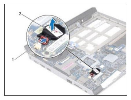
The coin-cell battery is glued to the system board. Using a plastic scribe, pry the coin-cell battery from the system board.
