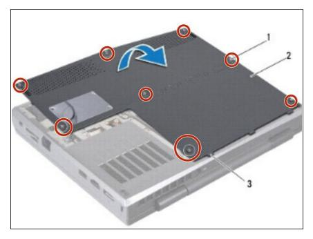
Tighten the eight screws that secure the base cover to the computer base.
