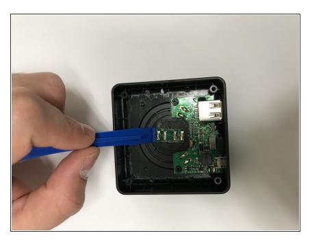
Use the plastic opening tool to carefully lift and remove the motherboard from the charging base.
