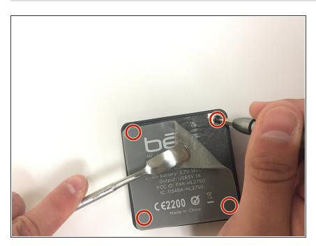
Use the screwdriver with the J0 bit attatched to detach all four 10 mm screws from the charging base.
