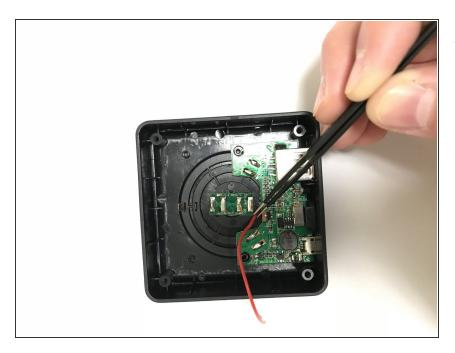
Use the tweezers to remove the red wire attached to the motherboard.
