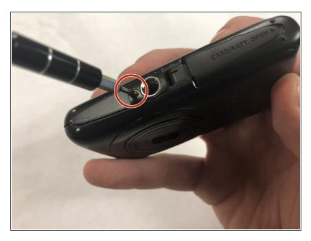
Remove the 4.0 mm Phillips screw located on the bottom of the camera.
