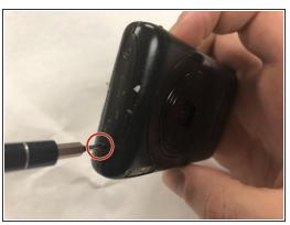
Remove the four 2.0 mm Phillips screws of the camera using the J00 bit from the 54-bit Driver Kit.
