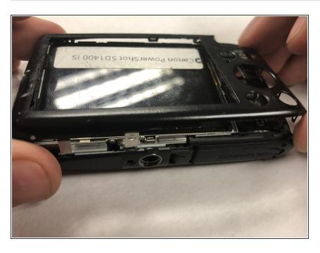
Remove the rear panel of the camera by hand using firm pressure.
