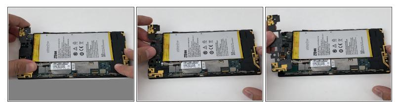
• Remove the top plastic motherboard cover using a plastic opening tool.
