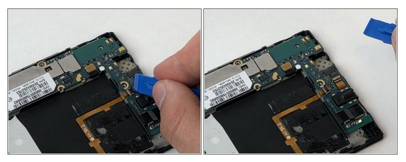
• Use a plastic opening tool to flip up the retaining flap on the volume ribbon cable <u>ZIF</u> socket.
