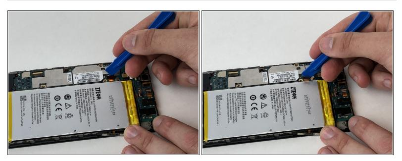
• Disconnect the battery cable from the motherboard with a plastic opening tool.
