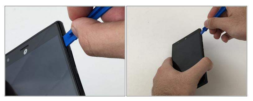
• Use an iFixit opening tool to separate the back from the device.
