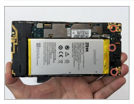
Remove the three 1.6mm Phillips #0 screws from the plastic cover on the motherboard.
