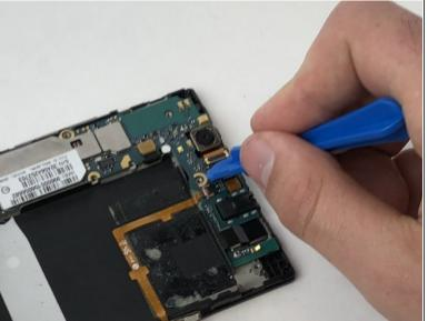
Using a plastic opening tool, disconnect the camera from the motherboard.
