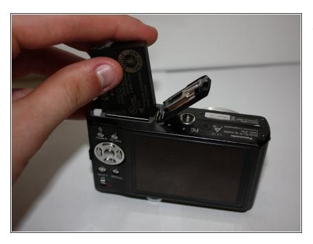
Remove the battery and the SD card.
