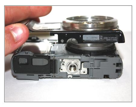
Carefully separate the front of the camera from the main body.
