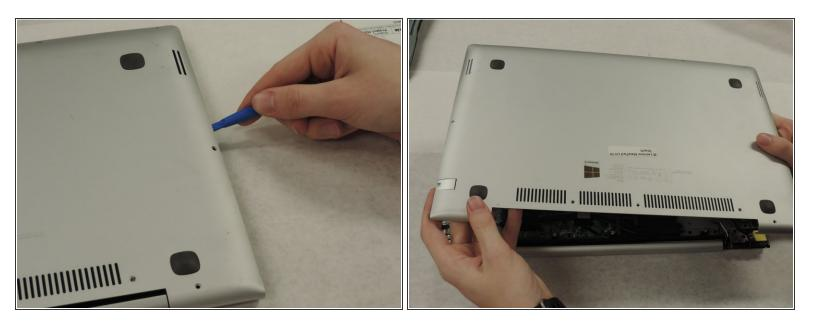
• To remove the panel, use a plastic opening tool to prevent any damage.
