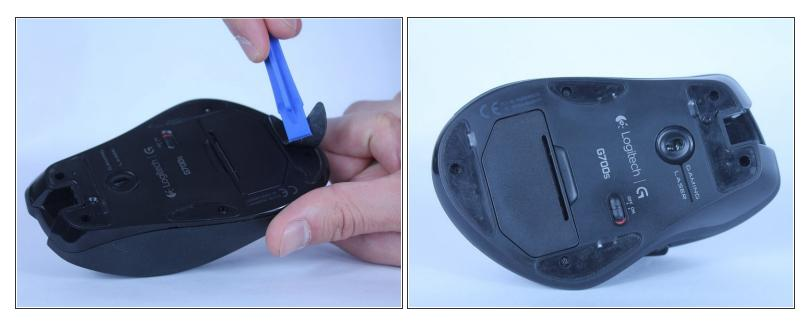
• Use a plastic opening tool to peel up the four skates from the bottom of the mouse.
