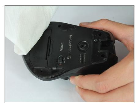
Using a towel with isopropyl alcohol, remove the old glue left behind from the removed skates.
