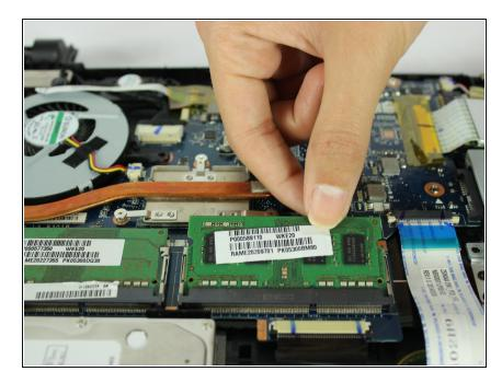
Pull the RAM out of the socket to remove.
