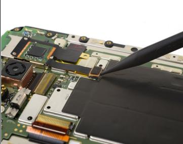
• Use the point of a spudger to lift the second display connector straight up and out of its socket.
