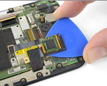
• Slide an opening pick under the PCB to slice through its adhesive and separate it from the SIM card slot.
