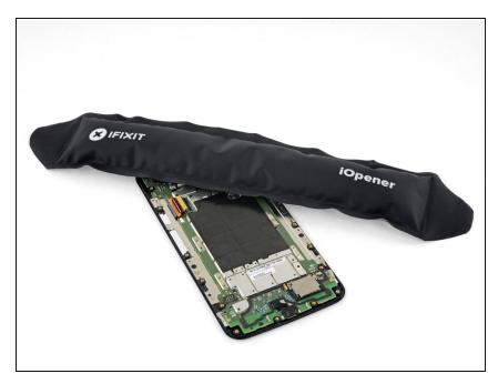
Prepare an iOpener and apply it to the small PCB adhered to the top of the SIM card slot.
