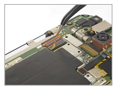
Remove the tape covering the display cable connector.
