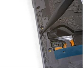
Use the point of a spudger to push the small clip securing the left side of the midframe toward the edge of the phone, releasing the clip.
