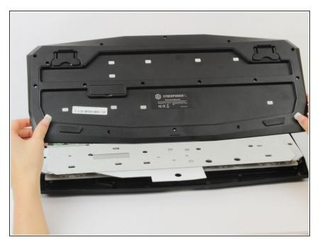
• Lift up and remove the plastic casing.
