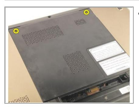
Loosen the screws that secure the memory door.
