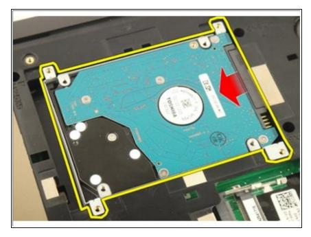
Slide the hard drive module in the direction shown in the image below.
