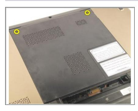
Loosen the screws that secure the memory door.
