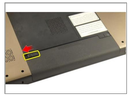
• Slide the release latches to unlock the battery.
