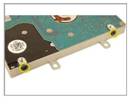
Remove the screws that secure the hard-drive bracket.
