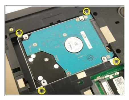
Remove the screws that secure the hard-drive bracket.
