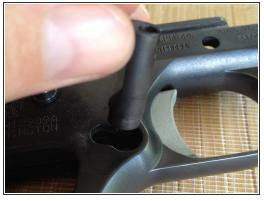
While pressing on the magazine release, use a small flathead (or the narrow angled edge of your leaf spring from the grip, it was designed with this purpose in mind) and turn the screw 90 degrees and it will pop loose for removal.
