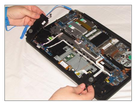
• Remove the speakers by picking the left and right pieces up and lifting them up and out of the computer.
