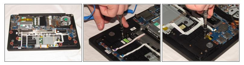
• Remove six 5.75mm Phillips #00 screws from the speakers.
