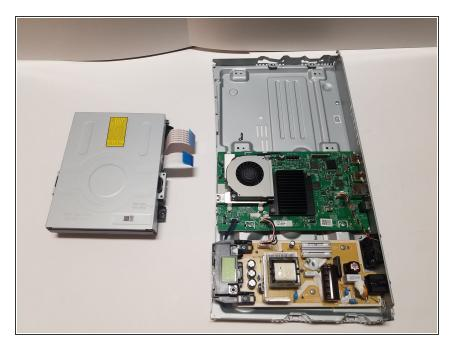
Once the connections are unplugged and the screws are removed, the disk drive can be lifted out. The previous steps can be done in the reverse order to replace the part.
