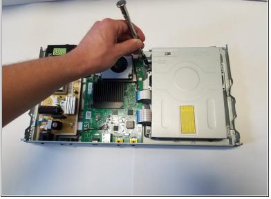
The disk drive has four 6.5mm screws located near each of its corners that hold it onto the frame.
