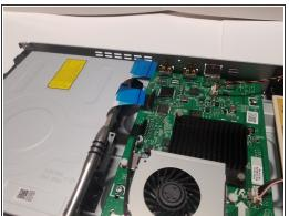
The disk drive has two connections to the motherboard that can be disconnected by pulling on the blue plastic tabs.
