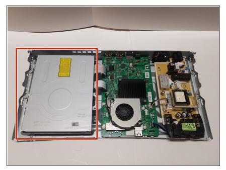
The disk drive is the large metallic rectangular unit that occupies a third of the space inside the unit.
