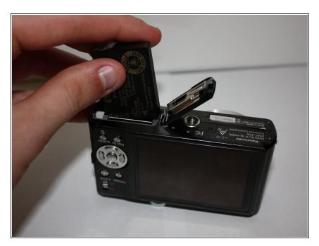
Remove the battery and the SD card.
