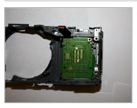
Carefully lift the SD card reader assembly out of place.
