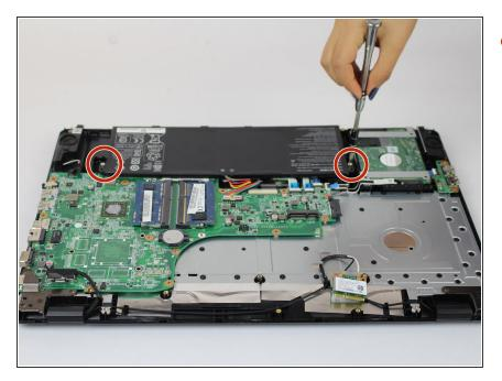
Remove the two 6mm Phillips #0 screws from the battery.
