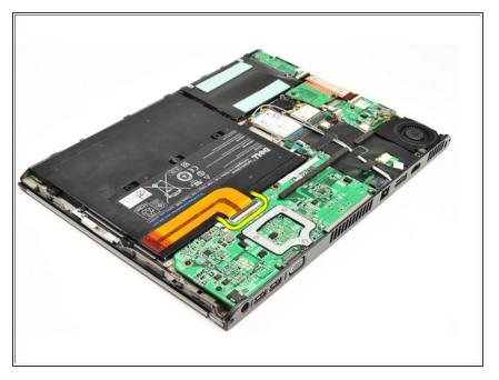
Lift the black cable-release clip to release the battery cable from the connector on the system board and disconnect the battery cable.
