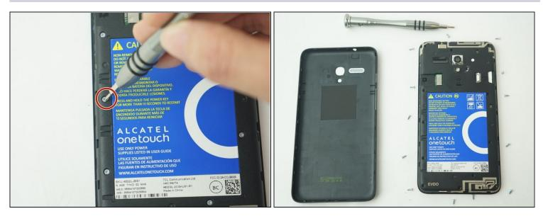
• Remove the 13 1 mm Phillips screws with JIS #000 Screwdriver.
