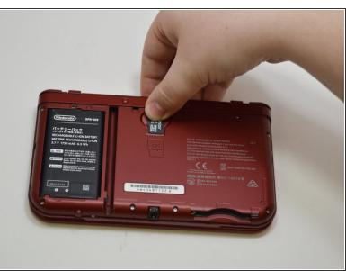
Remove the microSD card by pushing it in, the card should automatically pop out.
