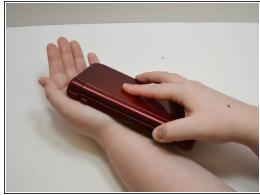
• To remove the battery, hold the device with the battery facing up in one hand, with a finger securely gripping the lid of the device, and gently flip the device over to your other hand. The battery should fall into your hand.
