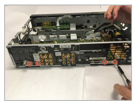
Remove four 1/2 inch screws using a nutdriver.
