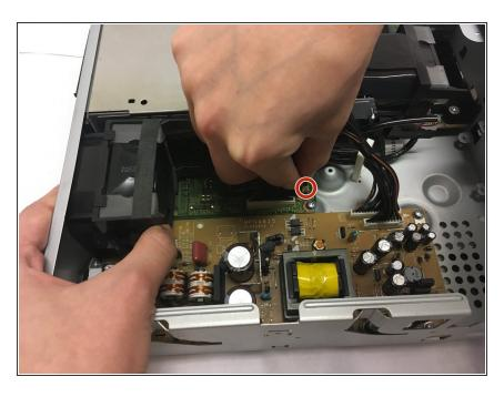
To replace the back cooling fan, grip the ribbon connector at slot M10 and remove by gently pulling upward.
