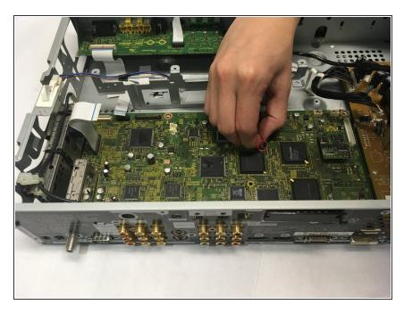
Pinch the securing tabs and lift the motherboard toward the interior of the device to remove it.
