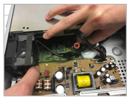
To remove the optical drive cooling fan, grip the ribbon connector at M11 and gently remove by pulling away for the slot.
