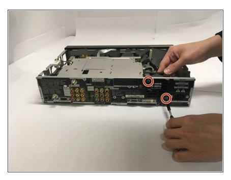
Remove the two 6.5 mm Phillips mounting screws at the back of the device.
