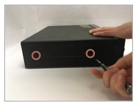
Remove the two 6.4 mm Phillips screws on each side of the device's casing.
