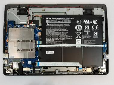
Insert a plastic opening tool under the bottom cover and slid it around the perimeter until all of the clips release.
