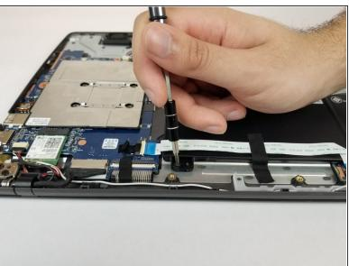
Remove the two 5mm Phillips #0 screws from the battery.
