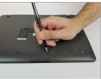
Remove the ten 7mm Phillips #0 screws from the bottom.
