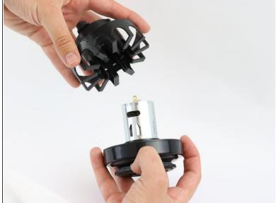
Twist and pull black casing off of the motor, leaving the motor and irremovable black impeller housing. To reassemble your device, follow these instructions in reverse order.
