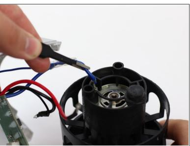
Use plastic spudger to remove blue wire from motor, freeing the motor.
