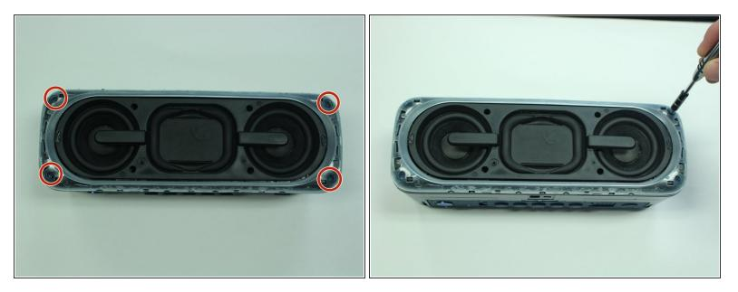
Once you have removed the outer blue casing, four T-8 screws (15 mm long) will be revealed on each corner. After removing these screws, simply pull the top part of the speaker way from the body to get the the inner part of the speaker.
