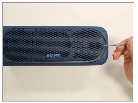
Remove the speaker case from the outer casing by prying it from the base of the speaker using a metal spudger.
