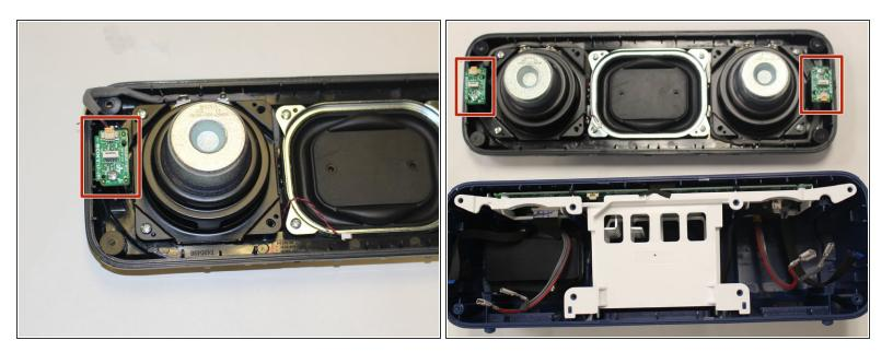
After you take the speaker plate off the body of the speaker, locate the LED control panels on each end of the speaker plate.
