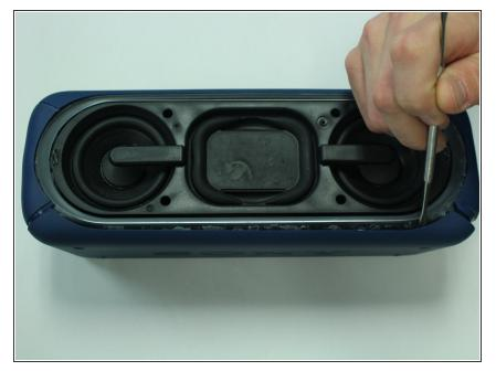
Pry the two rubber end pieces loose enough to pry off two pieces of the long plastic casing from the speaker body using a metal spudger.
