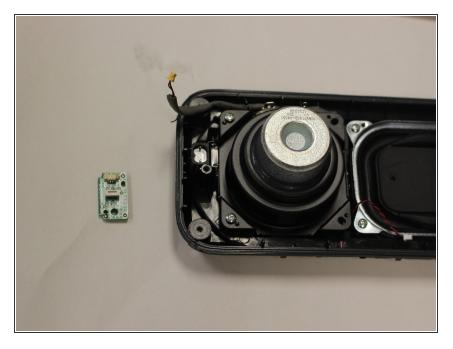
• Your LED light control panel is now disassembled and ready to replace.
