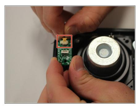
Carefully unplug the wire from the panel, releasing the panel from the speaker plate.
