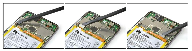
• Use the flat end of a spudger to disconnect the volume and power button, the display and the main flex cable.
