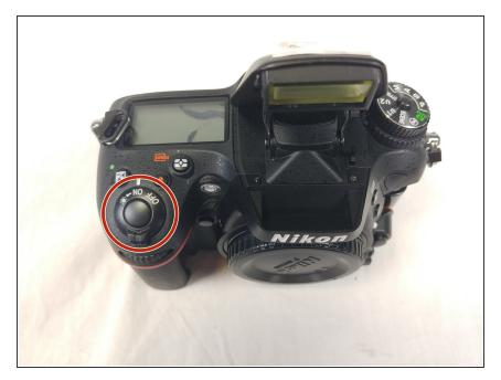
Turn the power off on the camera by turning the power dial.
