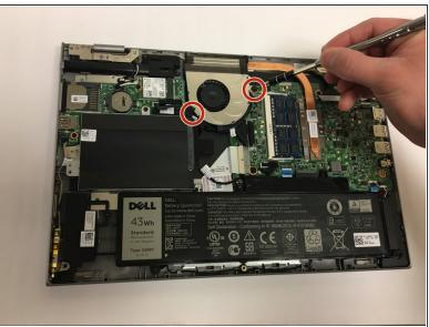
Unscrew and remove the 2 of the 7mm Phillips head screws holding the cooling fan in place.
