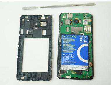
Gently pry off the Mid frame from the phone using a Metal Spudger.
