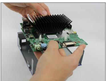
Lift the motherboard out of the casing.
