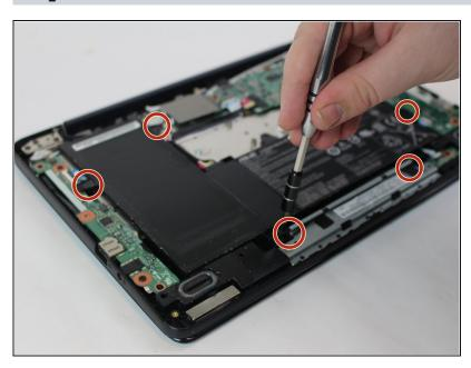
Unscrew the battery from the motherboard using a J000 screwdriver on the 3mm screws.
