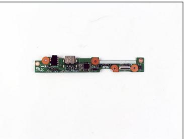
• Remove the final connections from the IO board with tweezers.
