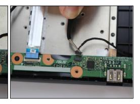
• After unscrewing, gently unplug all the connections to the IO Board with <u>tweezers</u>. We have highlighted where these connections are located in our images.
