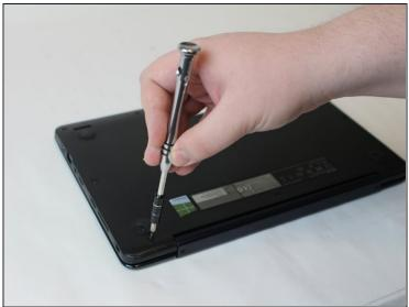
Remove the back 6mm and 8mm screws with a J000 screwdriver.
